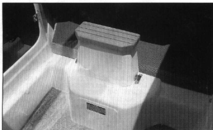
Photo 27 Cabin entry step and valve cover
