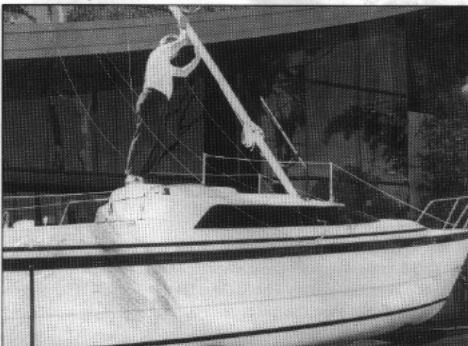
Photo 18 Lifting the mast
